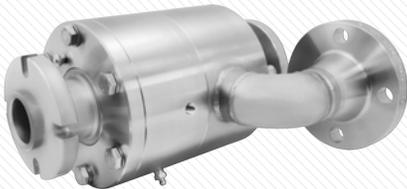
**Specialized Example 1** - designed for solid-liquid separation equipment for a pharmaceutical application. Features include specialized mechanical seals for -65° C, all stainless steel construction, and low temperature bearing grease.
