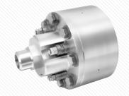
**Specialized Example 2** - designed to provide rotational movement to collector piping in a parabolic trough concentrated solar power (CSP) field. Features include a high temperature packing sealing system (1,000° F), internal corrosion-resistant bearings, and a design for direct welding to the piping system.
